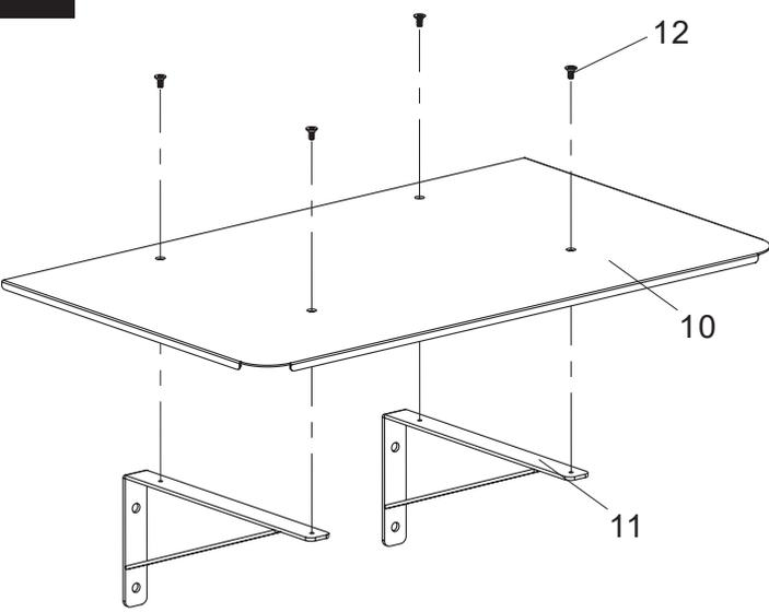
Diagram showing the top panel (10) being attached to the base frame using screws (12) and brackets (11).
