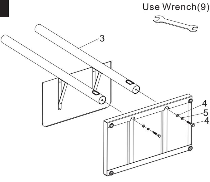
Diagram showing the top bar (3) being attached to the side panel (7) using a wrench (9) and screws (4, 5).
