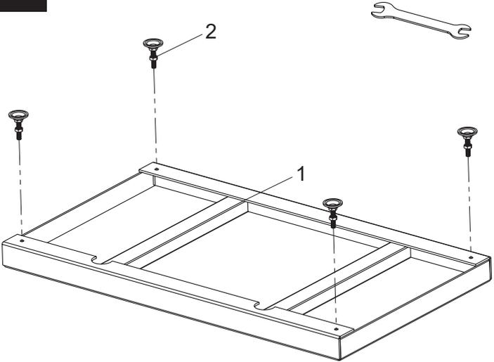
Diagram showing the base frame (1) being secured with screws (2) using a wrench (9).
